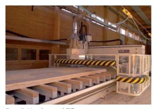
*Figure 3:* Manufacture of CLT (Courtesy of KLH)
